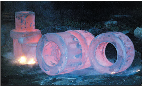
Forged Cylinders Being Air Cooled After Heat Treatment
