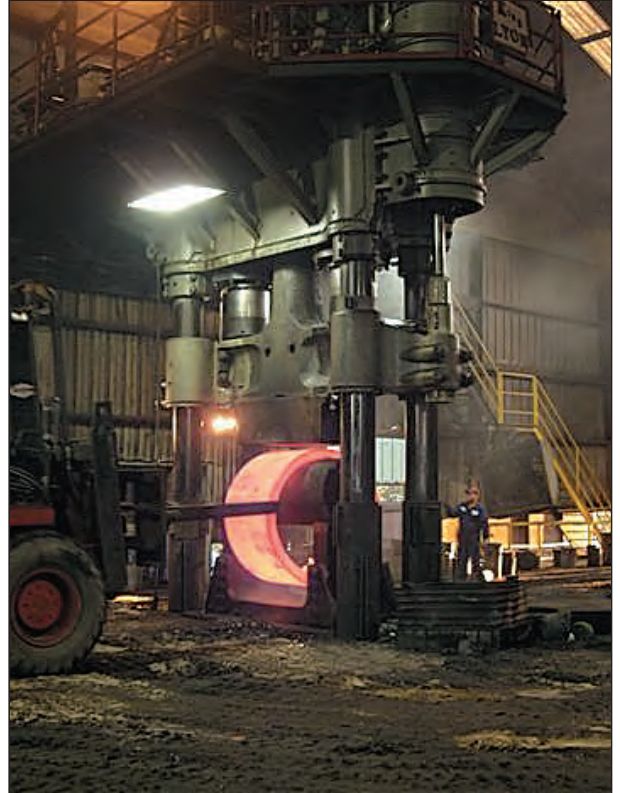
2500 Ton Press Forging Large Cylinder
