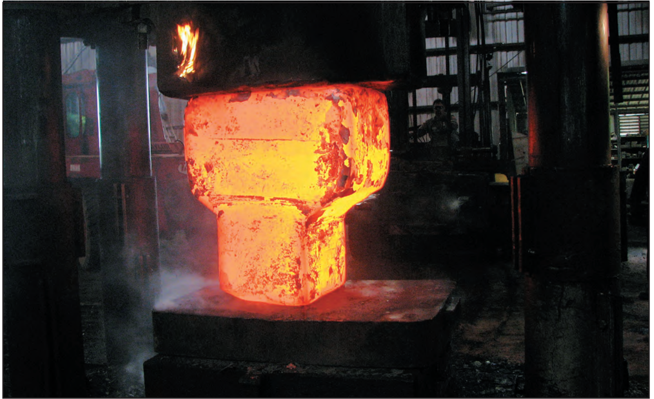
19,000 Lb Pigable Y Block Forging
