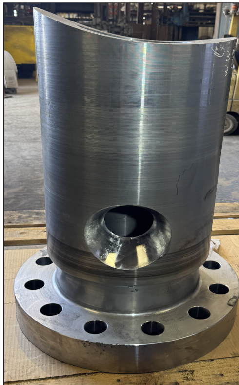
Hillside Contour with Pre-fabricated Outlet prep.
