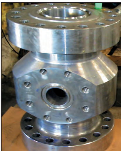
7 1/16" 15M Spool with 4 1/16" 15M Studded Outlets API PSL-3
