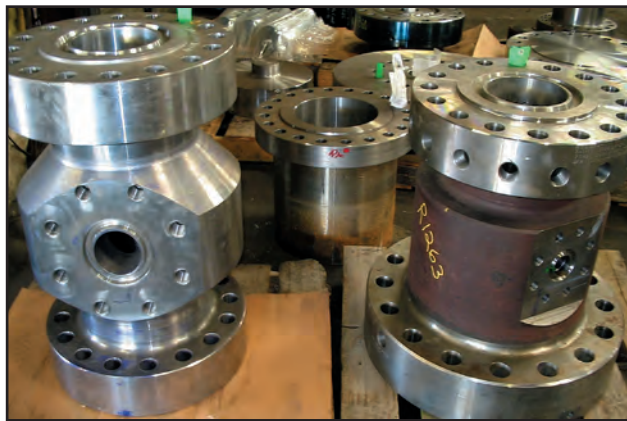
15M and 10M Spool with Studed Outlets
