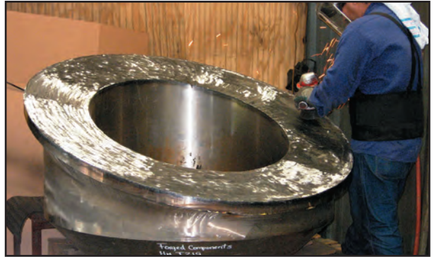
36" F11 Hillside Q-Lip Stubs for Coker Vessels
